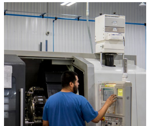
Model 300 Mist Collector installed on a CNC machine
