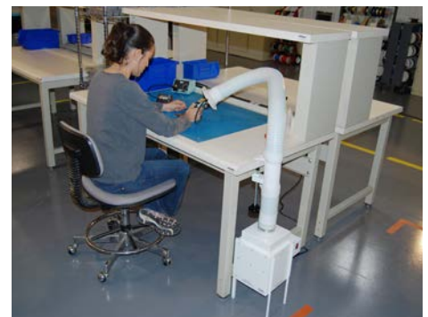
The Snorkel Sentry can easily be placed on the floor to free up valuable benchtop space.
